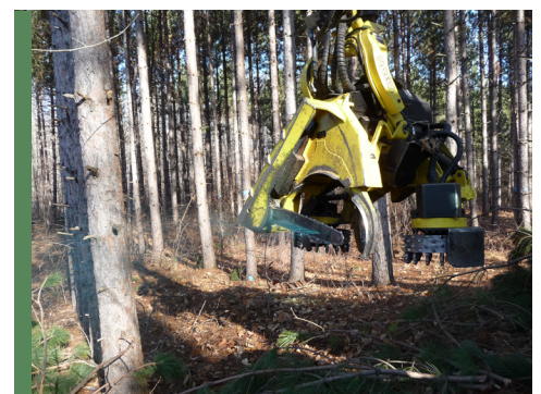
Pesticide solution is applied on fresh cut stumps through a perforated sawbar on a dangle head processor at the time of harvesting (blue dye is added as a visual cue to ensure acceptable coverage).
