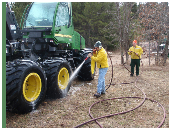
Clean logging equipment (tires, cutting head, etc.) with pressurized water prior to leaving HRD infested stands to minimize the risk of the spread of H. irregulare to a new location.
