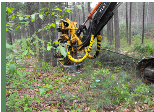
Pesticide solution is applied on fresh cut stumps through a spray nozzle attached on a fixed head processor (blue dye is added as a visual cue to ensure acceptable coverage).
