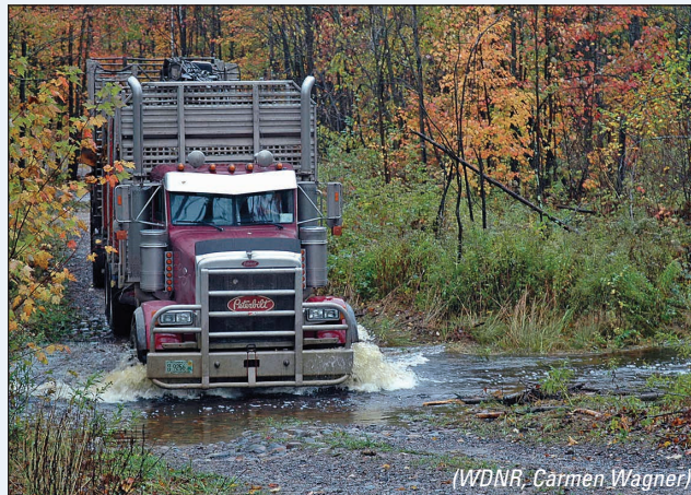
Figure 12-12: Fords are best suited to streams with a firm rock or gravel base.
