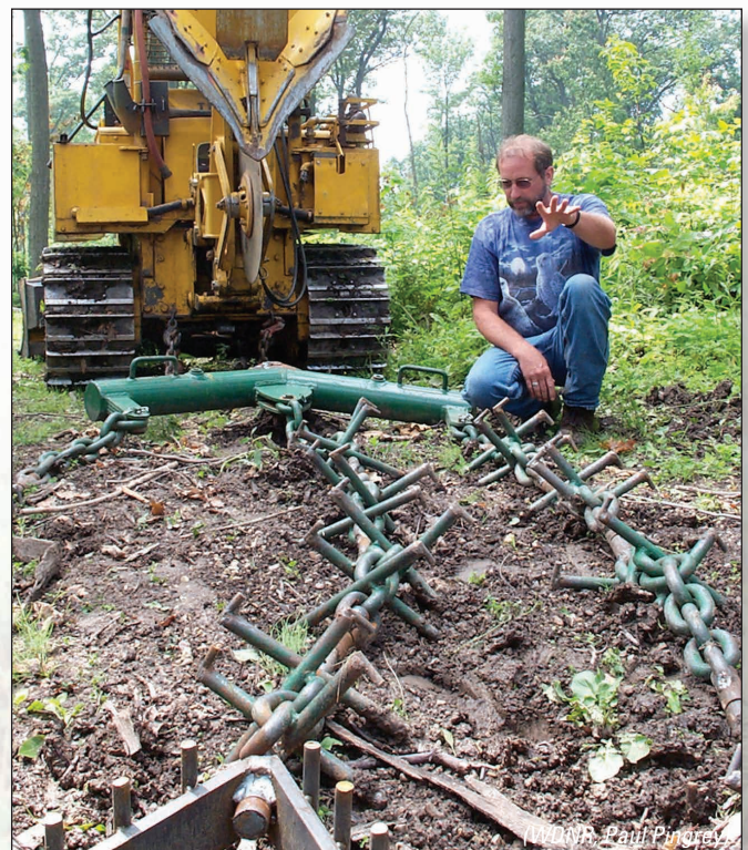
Figure 15-8: Soil scarification with a spiked anchor chain is a type of mechanical site preparation that prepares a seed bed for acorns in oak forests.
