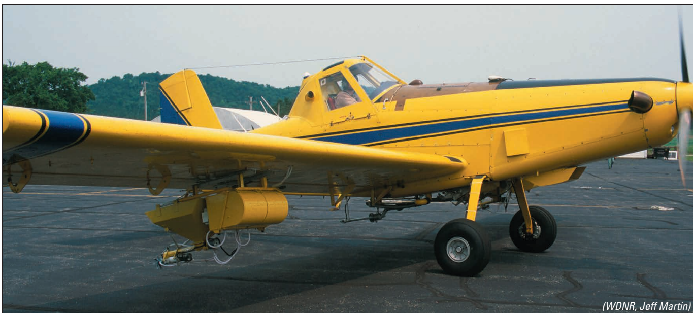
Figure 14-1: A spray plane equipped with special wing-mounted hoppers for dispensing Pheromone Flakes mixed with glue to control the spread of gypsy moths.
