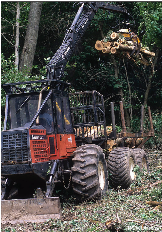
Figure 7-3: Tracked vehicles or vehicles with oversized tires like the one pictured above, have lower ground pressure and can help limit the negative impact on soils that compaction or rutting would cause.
