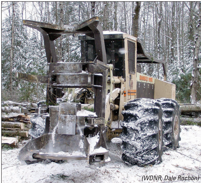
Figure 13-22: A feller buncher in Douglas County.
