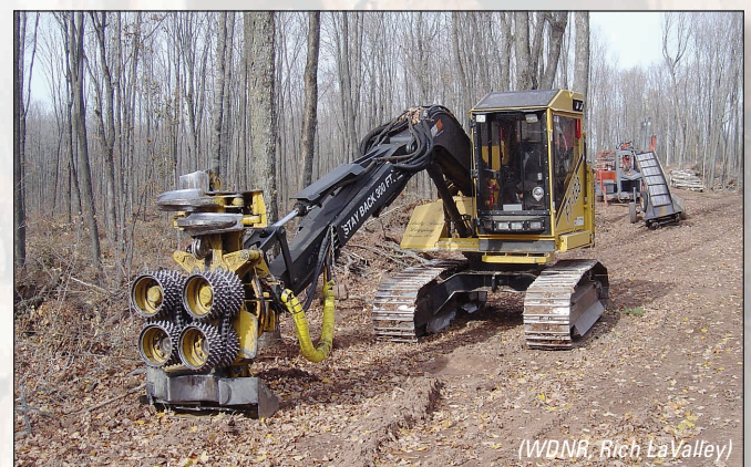
Figure 13-23: A processor in Iron County.
