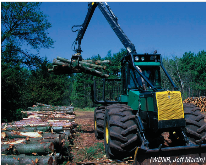
Figure 13-31: A forwarder offloads pulpwood at a woods landing. Forest management objectives may influence your equipment choice. Forwarders carry wood, thus causing little soil disturbance. Skidders scarify the soil by dragging trees or logs – a plus for natural regeneration where erosion is not a problem.
