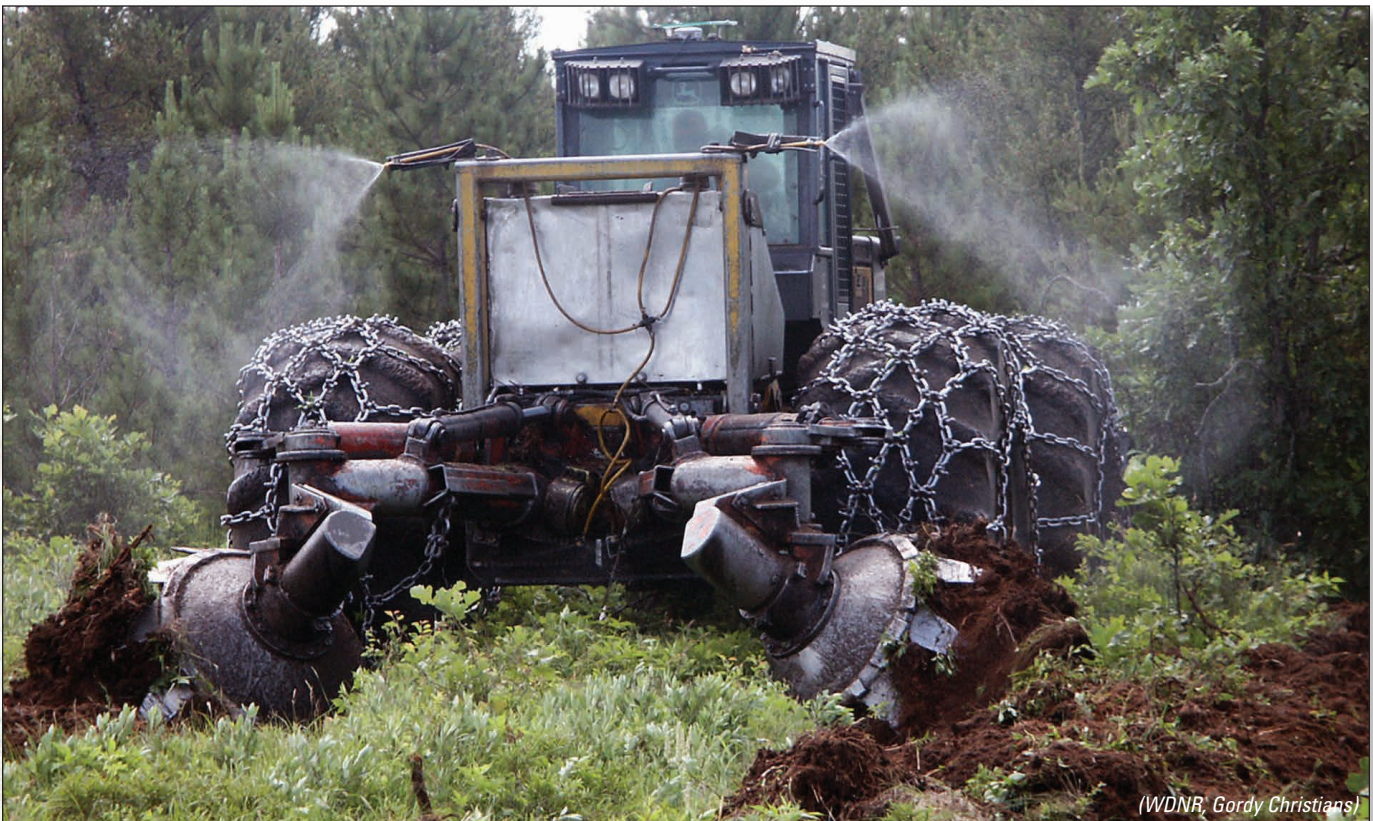
Figure 15-10: A disk trencher provides row scarification to prepare a harvested area for tree planting or direct seeding. Patch or row scarification methods like this one reduce competition for the new tree seedlings while minimizing soil disturbance on the site. Here, the mechanical and chemical site preparation are combined in one operation nine months prior to spring hand planting.
