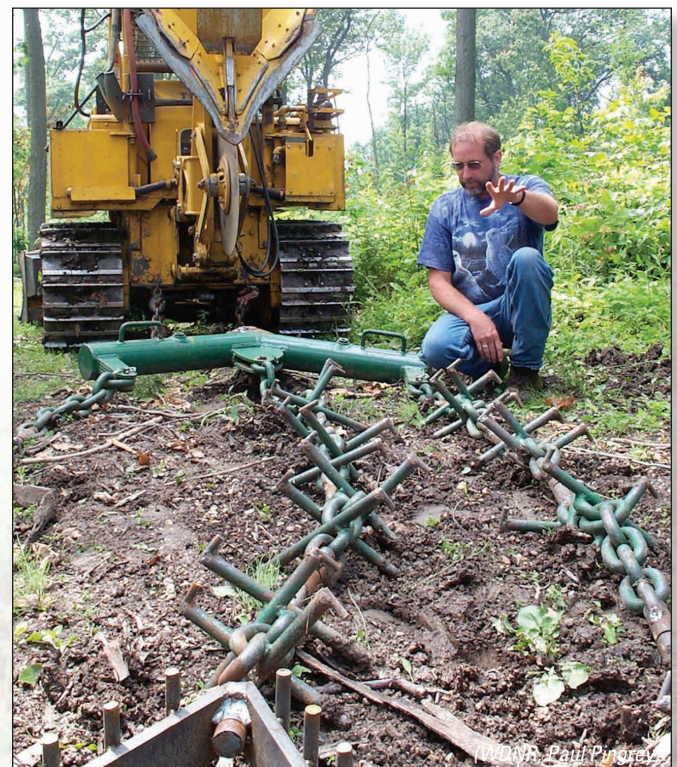
Figure 15-8: Soil scarification with a spiked anchor chain is a type of mechanical site preparation that prepares a seed bed for acorns in oak forests.
