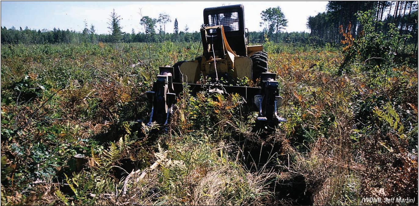
Figure 15-9: A Two-row Leno scarifier set up to create scarified patches in a clearcut. This approach causes minimal site disturbance, yet provides exposed soil for ideal planting conditions.
